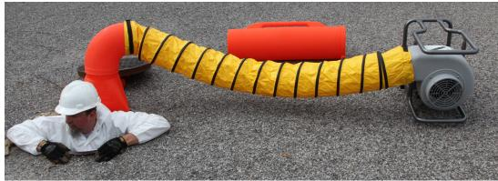
The Saddle Vent® allows unrestricted entry and exit and improves ambient light in a confined space opening.
