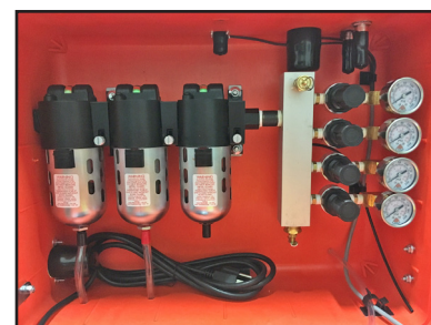
Breather Box® with 4 Independent Regulators BB50-CO4R
