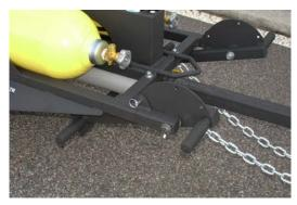
**STEP 10)** Pull pins, rotate handle bars to underside of cart and re-pin.
