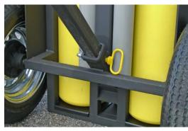
**STEP 1)** Remove retaining pin.
