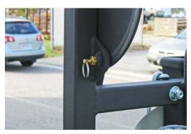
**STEP 4)** Pull spring loaded pin.
