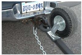
**STEP 9)** Couple to tow vehicle and attach safety chains.
