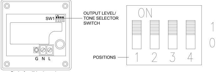
Back of audible alarm when removed from alarm enclosure.
