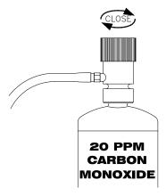
The monitor is now calibrated and should be recalibrated monthly or if accuracy is questionable. Check local requirements and recalibrate as required.
