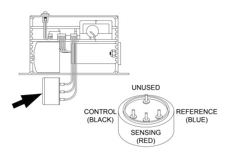
Step 4) Remove sensor from sensor cup and remove leads. Take the new sensor and remove the metal spring. Reattach leads to the proper colored terminals on the new sensor. Install new sensor into sensor cup.
