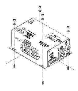
Step 5) Reassemble monitor and reinstall in unit. Connect all cables and air sample hose. Allow monitor to stabilize 30 minutes to 1 hour and recalibrate.
