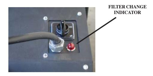
If this light actuates, change the pre-filter pad. <u>Every 8 hours, inspect the pre-filter pad and replace if clogged</u>. <u>If the red light stays on after replacing the pre-filter, the HEPA filter should be replaced</u>.
