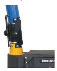
Remove the screws and place the arm over the inlet aligning the mounting holes to the cabinet. The piston will always be placed toward the front of the cabinet as shown in the picture above. Install the six screws and securely tighten the arm to the cabinet. The unit is now ready for use.
