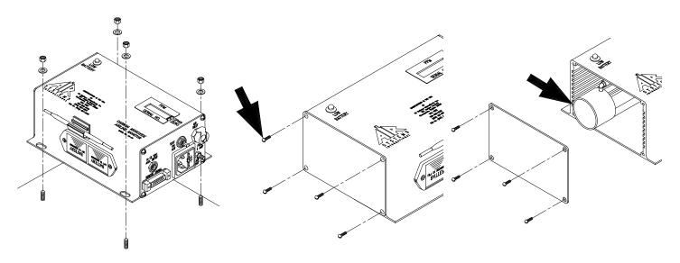
Step 1) Disconnect all external connections. Remove CO monitor from the unit.
