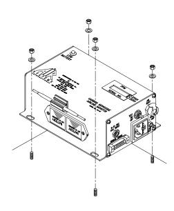
Step 5) Reassemble monitor and reinstall in unit. Connect all cables and air sample hose. Allow monitor to stabilize 30 minutes to 1 hour and recalibrate.
