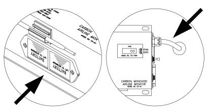
**Note:** The 9 volt batteries continuously provide a required bias voltage to the CO sensor and power the monitor. If power is removed for a period of 2 hours or more, a 1 hour restabilization period is required for the sensor as erratic readings may occur.
